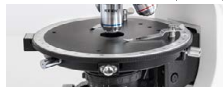
Center-adjustable and turnable polarisation stage
