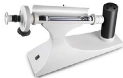
Cuvette in measuring chamber
